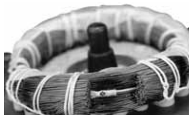
Fig. 26 PTC sensor incorporated in winding
