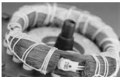
Fig. 28 Thermal switch incorporated in winding
